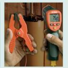
TP200 Type K clamp probe provides hands-free secure grip when measuring temperature on pipes up to 38mm (1.5") diameter
